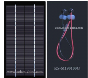
Item No. KS-M190100G 2W--18V/111mA Dimension: 190×100×5mm Tempered glass Solar Panel
